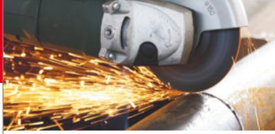
PIPELINER is the cutting, grinding and beveling range designed for pipes fitting, notching and welding preparation.
