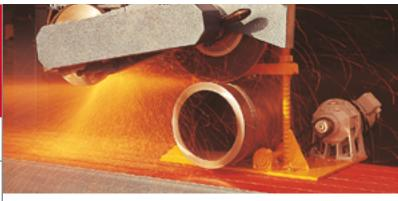
We produce a wide variety of hardness grades, diameters, thickness and bore sizes, peripheral speed in order to adapt to every kind of existing machine.
