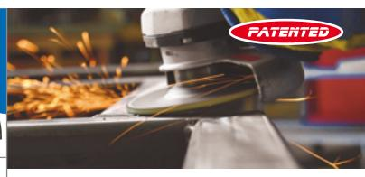
TURBOTWISTER is the semi-flexible wheel, covered by patent, for grinding and finishing of internal and external curved surfaces, characterized by a working surface with rhomboidal grooves that increase removal rate and create a cooling effect thanks to air circulation through the grooves. The specification for metal, free from iron, sulphur and chlorine compounds, is also suitable for stainless steel. The large contact area guarantees an excellent planarity of the surface treated.
