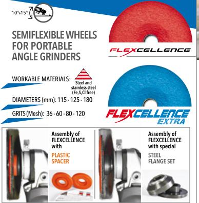
To get the best from FLEXCELLENCE and FLEXCELLENCE EXTRA, every package contains a thick flange (SPACER) specifically designed to position the wheel closer to the grinder safety guard profile allowing also flat grinding. For even more professional users GLÓBE supplies a special STEEL FLANGE SET that fits to all the grinders existing on the market and optimize the disc positioning.
