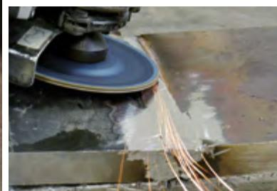
Specific applications of TurboTwister CERAMIC POWER in heavy carpentry: grinding of flat concave and convex surfaces.
