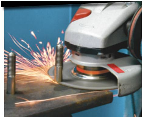
Thanks to the special "SPACER" and the depressed center shape, the machine shaft and the locknut do not protrude from the dome cavity, allowing to carry out flush cuts in a comfortable and safe position. The depressed center with metal reinforcement also confers more rigidity than a flat disc, allowing perfectly straight cuts.
