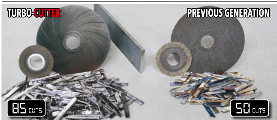
On the right: the final result of the comparative laboratory test on 2x1/4" mild steel bars with 125mm discs.
