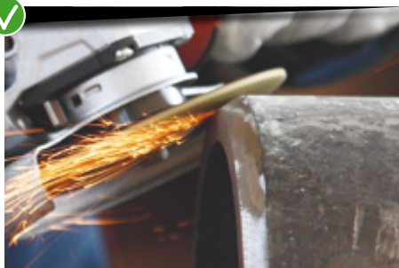
BEVEL OF SHARP EDGES
